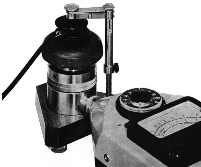
Fig. 2.4. Artificial Ear and Precision Sound Level Meter in combination.
